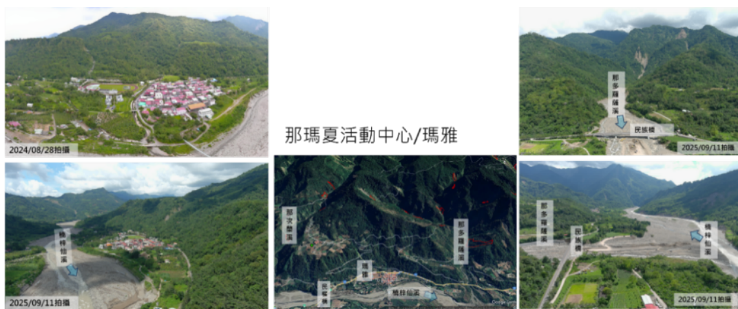
(c)瑪雅村、那多摩薩溪土石流出推擠旗山溪(楠梓仙溪)流心
